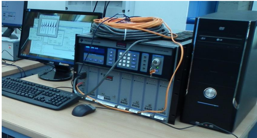
The multimanometer and the control and programming system
