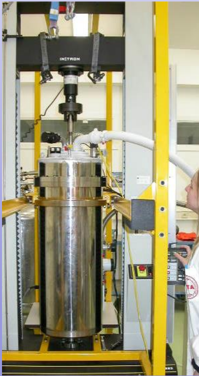
Universal testing machine with continuous flow cryostat
