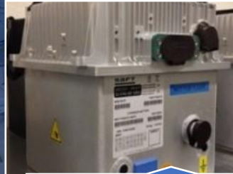
Battery / Super Capacitor
