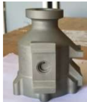
Components Scalmalloy (Aluminium) MA – C295/MRT AIRBUS
