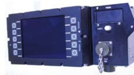
Figura 16-. Maintenance Data Panel (MDP).
